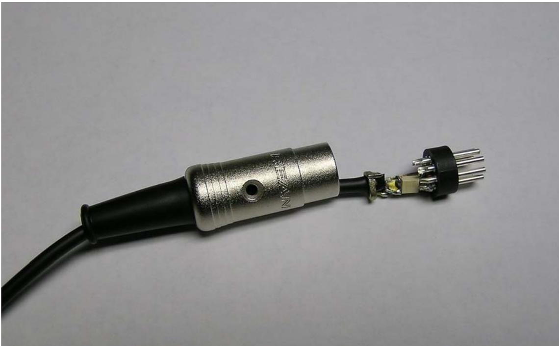
The Neutrik metal hood DIN connectors are very sturdy and they don't pull apart when you remove the plug from the radio. This is very common with the cheap plastic hood connectors. Even though this assembly is very sturdy and has a cable strain relief, I do not recommend that the DIN plug ever be removed by pulling on the cable. Pulling on the cable may place a strain on the solid state switch possibly breaking off a lead.
