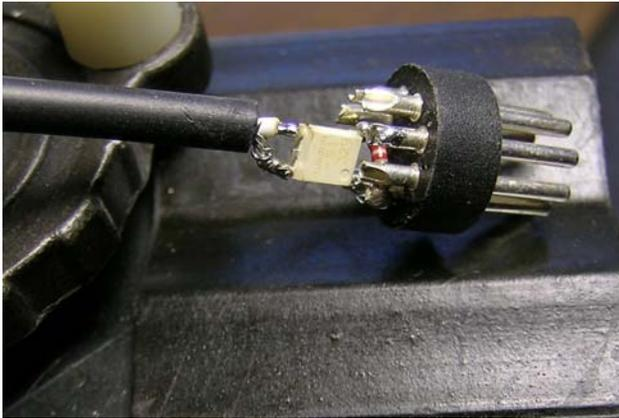
Here is a photograph of the final assembly just prior to sliding the metal hood over the connector. I found that some silicon bath tub caulk squirted into the rubber boot after the hood is in place will provide an additional strain relief and make the assembly more robust.
