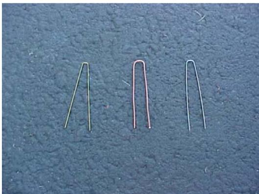
**Left - staple made of small diameter brass tubing**
